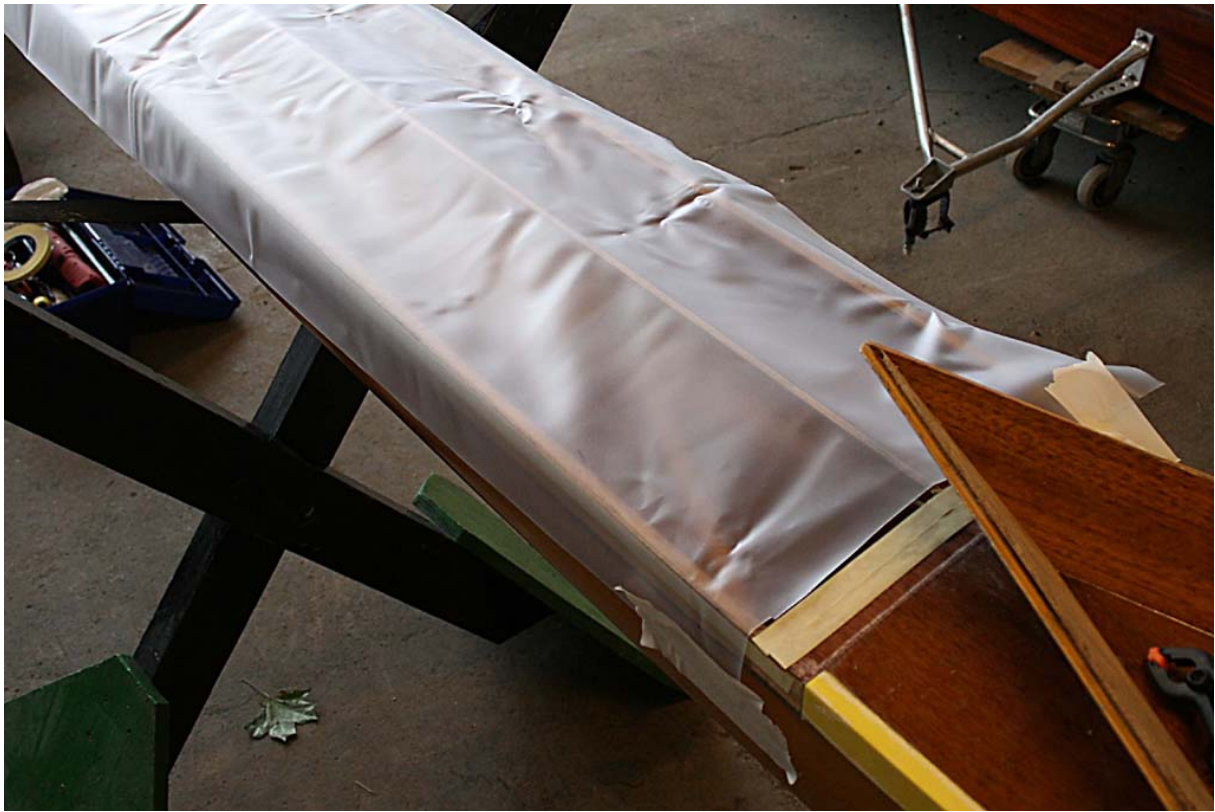
Figure 6: Laying the decking material over the deck in order to cut it to shape; see also the arrangement of transverse tape strips at the cockpit end of the deck.
