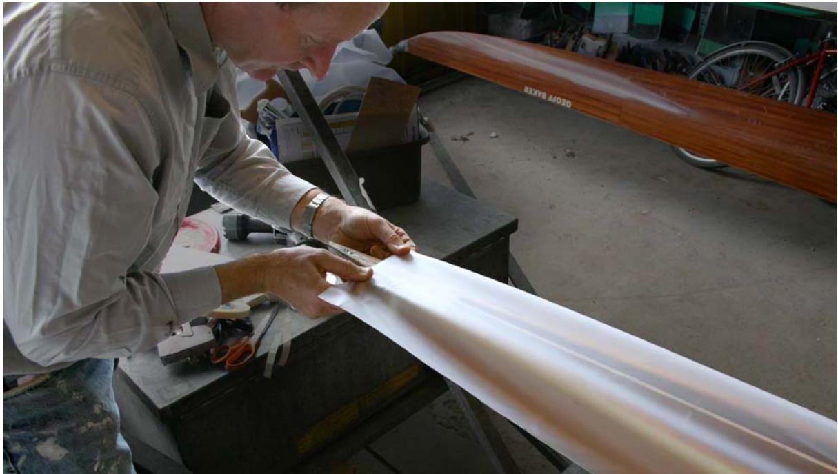
Figure 8: Stretching the decking material lengthwise; draw it out to the point you determined during your “practice” and press it down firmly onto the tape.
