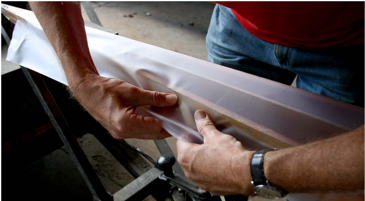
Figure 13: Another view of the transverse stretching. See the very slight wrinkles in the material beside both the boatman's thumbs, especially his right: this shows that not quite enough longitudinal tension has been applied. At this stage there is usually enough give in the joint to allow these wrinkles to be pulled out when the next section is stretched a moment or two later.
