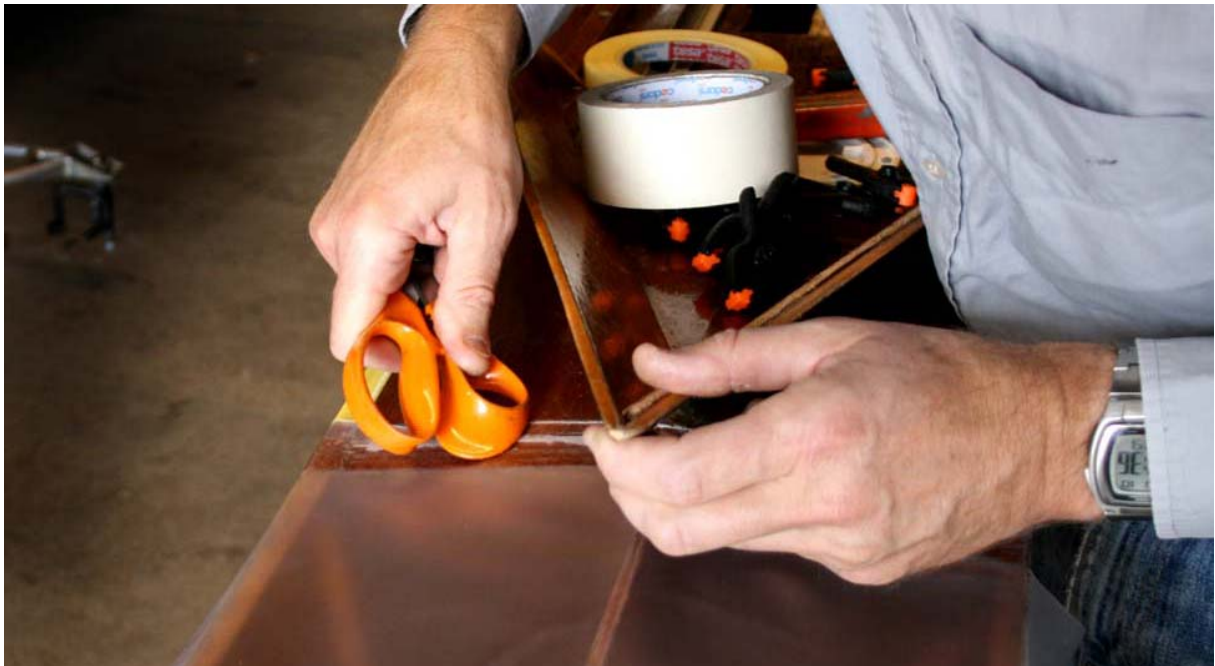
Figure 7: Rubbing down the first joint - the cockpit end of the deck - with the handle of the scissors to ensure maximum strength of the joint.
