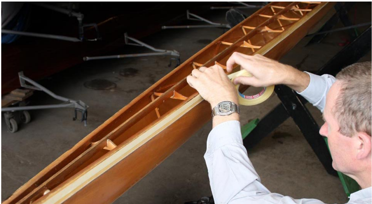
Figure 3: Applying double-sided tape to the sides of the hull
