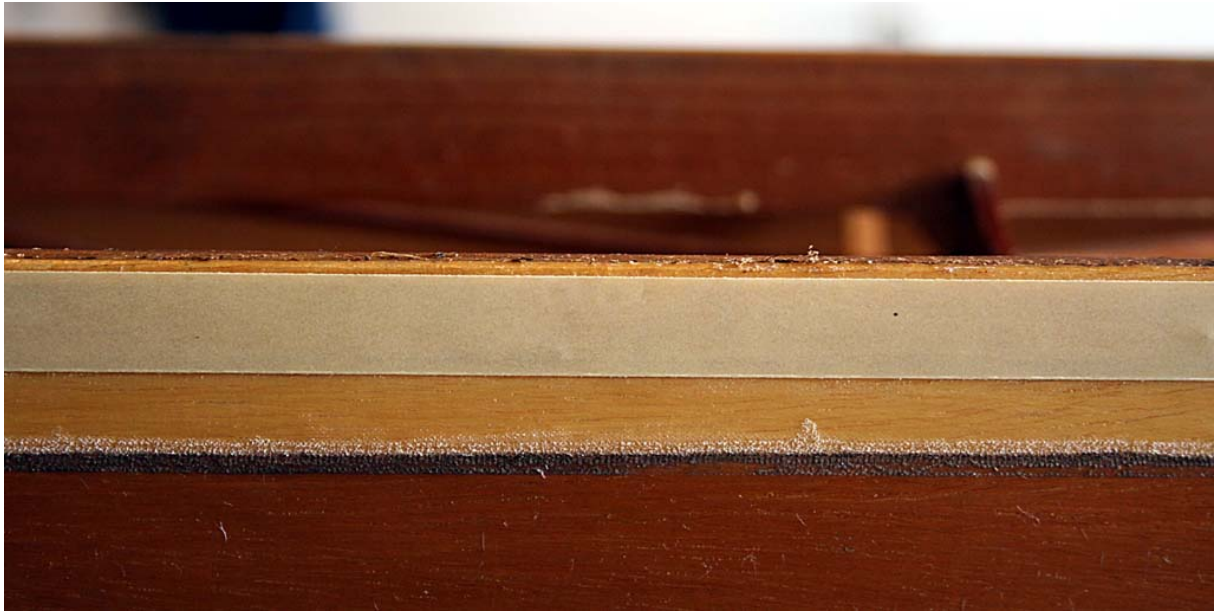
Figure 4: The tape applied, showing the approximately 1mm gap between the tape and the top of the hull. You can also see the residue from the original tape; a purist might try to remove it with a solvent of some kind.
