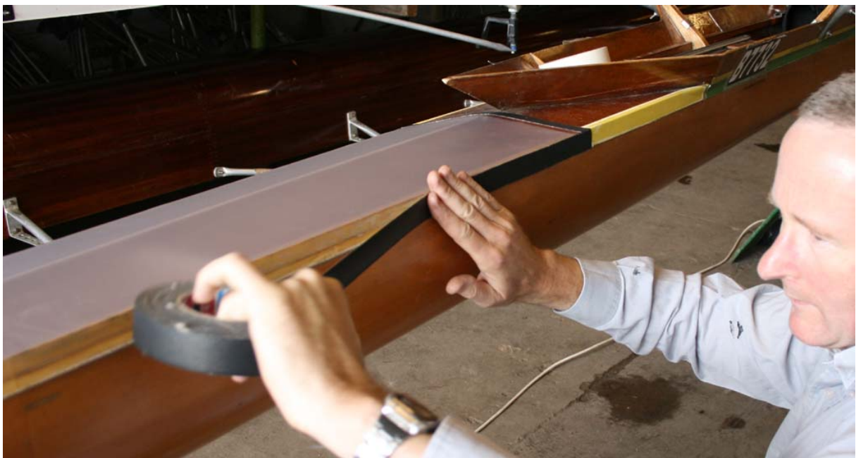
Figure 15: Applying binding tape.
