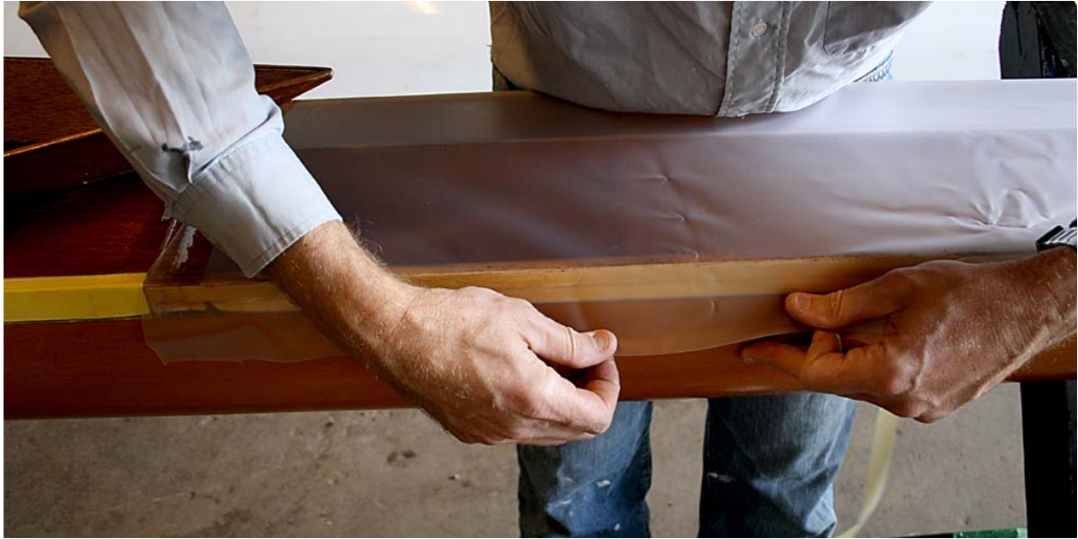
Figure 10: Stretching the first side of the canvas. The near side of the material is anchored by the boatman's body against the hull while slight tension is applied and the material pressed onto the tape.
