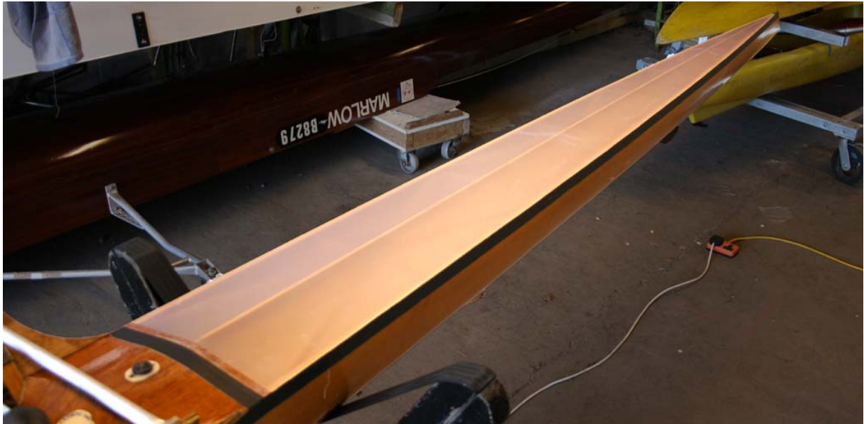
Figure 16: The finished deck. The slight creases in the material, left over from where it was folded for posting, can just be seen.
