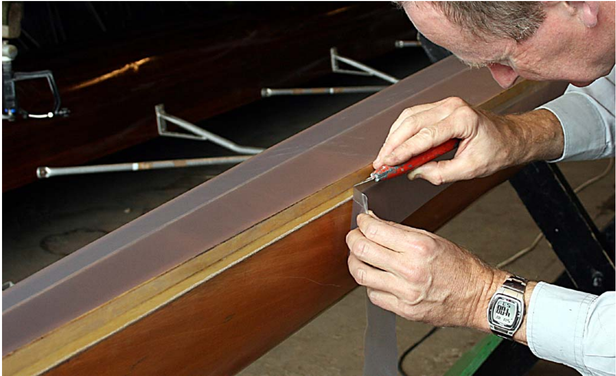
Figure 14: Trimming off the surplus tape along the side of the deck. With a really sharp blade it's possible to cut the plastic just enough that it comes away with a gentle pull, without touching the surface of the wood. The third and fourth fingers of the boatman's hand rest on top of the decking and serve as a guide while he runs the knife smoothly along the joint.
